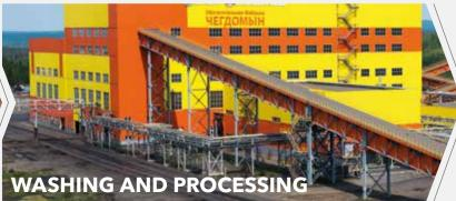
Washing plants and processing facilities adjacent to our mines and open pits improve the quality of our coal. Washing reduces ash, increases heat content and ultimately improves our coal's market value. The coal is also crushed and screened so that it can precisely meet customers' size specifications without affecting quality.
